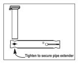
Thread the keyboard onto the extender pipe, turning until you hear a few clicks and feel slight resistance. Do Not Overtighten! Finger-tight is sufficient. Tightening beyond this point may make removal difficult.
