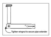
Thread the tray onto the extender pipe, turning until you hear a few clicks and feel slight resistance. **Do Not Overtighten!**Finger-tight is sufficient. Tightening beyond this point may make removal difficult.
